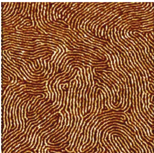
Figure 1 AFM image (phase contrast) of the neat Vector 4111 sample (2 \mu\text{m} scale).
